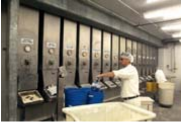
Jorge Javamillo scales micro-ingredients at the Bloomfield bakery. The bins are loaded one floor above, with distinct and separate loading systems for allergenic ingredients.
