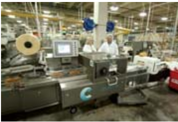
Project Engineer Marta Mulyk (left) and Project Manager Glenn Wright discuss optimization issues involving the plant's flow wrappers. The plant is the first North American bread installation for the high-speed packaging equipment.
