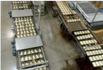
Raw dough is conveyed to and from a proofer. Significantly larger proofers were engineered for the plant compared to previous Pepperidge projects to enable the facility to achieve volume objectives.
